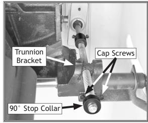
Figure 90. 90° stop collar and cap screws.
